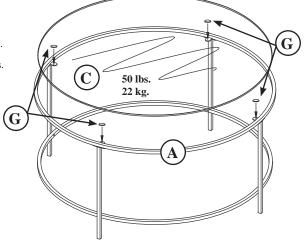
Stick the GLASS PADS (G) onto the TOP RING (A) as shown. Then, carefully set the GLASS TOP (C) onto the GLASS PADS.
