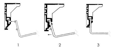
If extra space is needed to access sockets etc Basket may be moved to position 5 whilst access is required – Always return to position 3 when work completed
