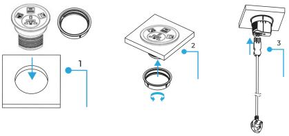
STEP 1. Remove the locking ring and place the module in the desk cutout.
