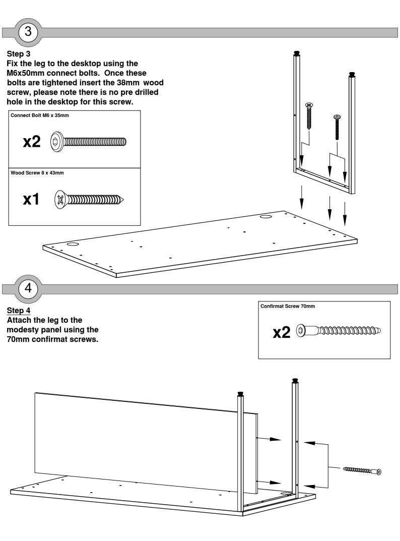
5 Confirmat Screw 70mm (Silver) Step 5 Attach the leg to the x2 🛈 modesty panel using the 70mm confirmat screws. 0**\_\_\_\_\_\_** 6 Wood Screw 8 x 43mm Connect Bolt M6x35mm Step 6 Fix the leg to the desktop **x2 x1** 貿 using the M6x50mm connect bolts. Once these bolts are tightened insert the 38mm wood screw, please note there is no pre drilled hole in the desktop for this screw.
