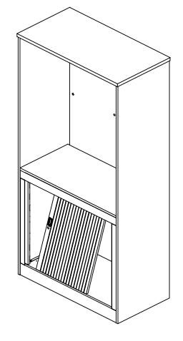
$\begin{tabular}{l} Step 4 \\ \hline Tilt towards LH whilst locating into the top track. \\ \hline Step 5 \\ \hline Keeping the shutter vertical, push into the open position. \end{tabular}$
