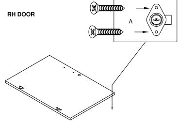
Fit the latch at the top hole when fitting full height doors.
