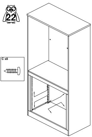
Screw the steel inners Z8T into place.
