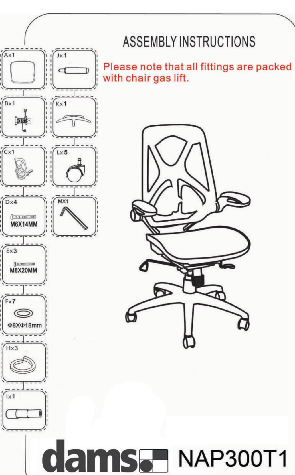
Do not tighten bolts fully until you have completed assembly.
