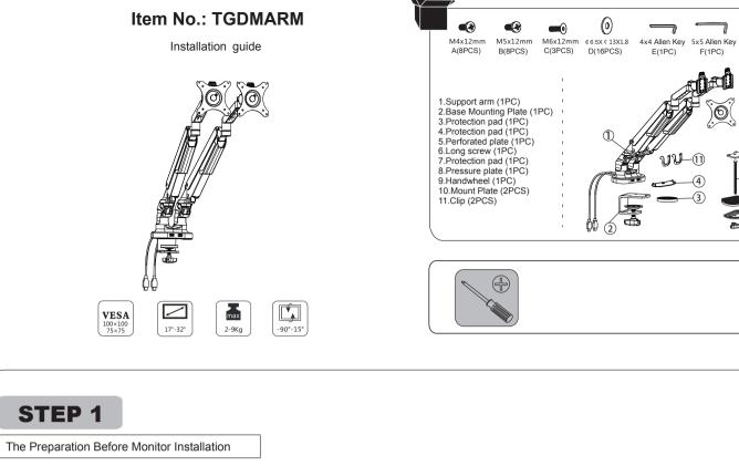
1.Make sure there are VESA holes 100x100mm or 75x75mm in the monitor. If not, cannot be installed. 2.Remove the original fixed base of monitor.Be careful not to scratch the screen.
