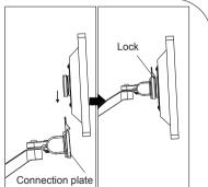
Hang the monitor on the plate from top to bottom and ensure it is tightened
